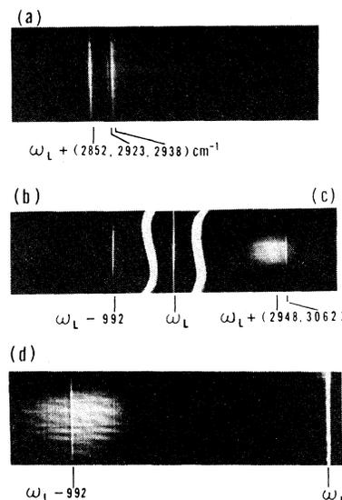
Fig. 2. Spectra taken with ASA-400 film, four pulses per exposure under polarization conditions described in text. Samples were (a) cyclohexane and (b)–(d) benzene. Asymmetric line shapes result from interference as described in the text. Structure appearing in background transmission in (c) and (d) is from spurious interfering reflections. The frequency of the narrow-band pump laser is marked  $\omega_L$ .
