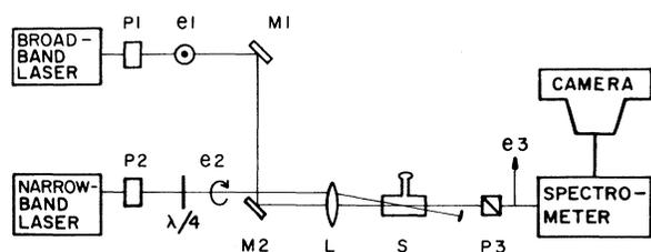
Fig. 1. Apparatus for observing Raman-induced Kerr effect. Glan polarizer  $P1$  produces probe polarization  $e1$ . Glan polarizer  $P2$  and mica  $\lambda/4$  plate produce pump polarization  $e2$ . Probe and pump beams are made to overlap over a region ( $\sim 8 \times 0.1 \times 0.1$  mm<sup>3</sup>) in sample  $S$  by mirrors  $M1$  and  $M2$  and a 25-cm focal-length lens  $L$ . Glan analyzer  $P3$  passes polarization  $e3$  into spectrometer.
