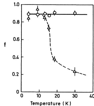
FIG. 2. Temperature dependence of the apparent Debye-Waller factor  $f$  of  $^{57}\text{Co}$  in Al. Upper curve circles,  $^{57}\text{Co}$  on substitutional site; lower curve triangles,  $^{57}\text{Co}$  with trapped single interstitial.
