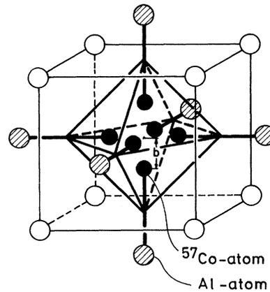
FIG. 3. Equivalent configurations for a mixed dumbbell, which can be formed by jumps of the <sup>57</sup>Co-impurity atom in the octahedral "cage" in a fcc lattice.
