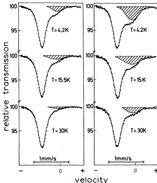
FIG. 1. Mössbauer spectra of  $\text{Al } ^{57}\text{Co}$  with the sample at various temperatures after two electron irradiation runs at about 100 K. Natural iron absorber at 77 K. Hatched: "defect line" corresponding to 17% (left side) and 36% (right side) of  $^{57}\text{Co}$  atoms with trapped interstitials.
