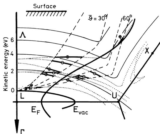
FIG. 3. Contours of constant energy for Cu characterizing direct optical transitions observable in the spectra shown in the upper portion of Figs. 1 and 2.
