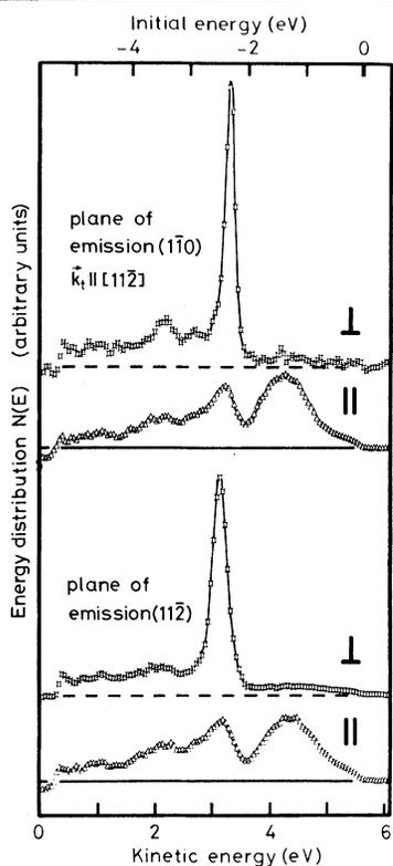
FIG. 1. Angular-resolved energy distribution of photoelectrons emitted from a Cu(111) surface at normal incidence of plane polarized light with 10.2-eV photon energy and  $\vartheta = 30^\circ \pm 7^\circ$ .
