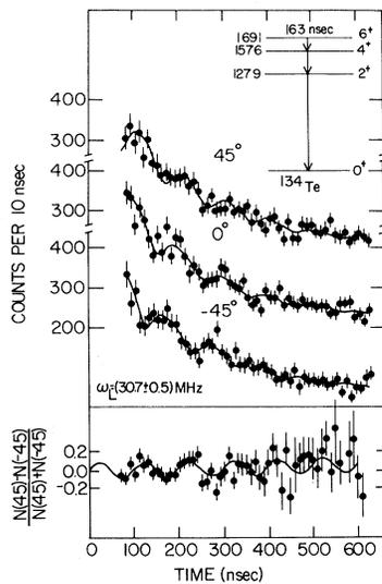
FIG. 2. Time spectra of the 115.3-keV radiation of  $^{134}\text{Te}$  at three angles with respect to the fission direction. Normalized differences between the intensities at  $45^\circ$  and  $-45^\circ$  are given in the lower part of the figure. The solid lines were obtained by a least-squares fit to the data. The decay scheme of  $^{134}\text{Te}$  as determined in Refs. 3, 4, and 5 is also shown.
