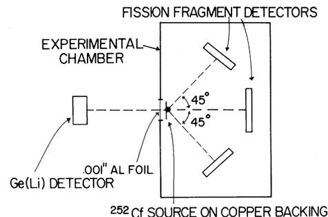
FIG. 1. Schematic description of the experimental system.
