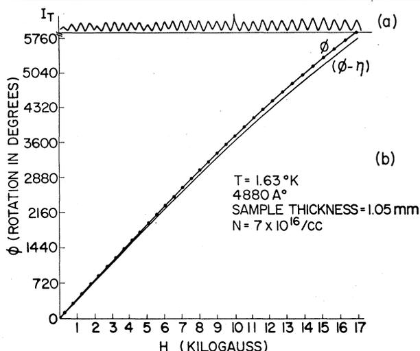
FIG. 2. (a) Transmitted intensity,  $I_T$ , versus  $H$  with fixed position of Polaroid analyzer. Separation between peaks corresponds to  $180^\circ$  of rotation. (b) Curve labeled  $\phi$  is plot of peaks in (a) and  $\phi - \eta$  is spin FR.
