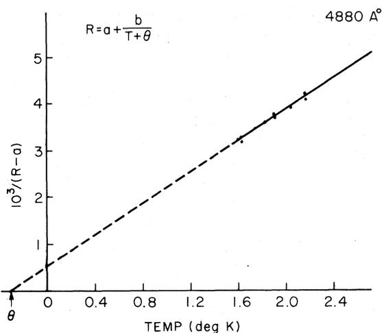
FIG. 3. Reciprocal of spin rotation,  $1/(R-a)$ , versus  $T$  showing extrapolated Curie-Weiss constant,  $\Theta = 0.3 \pm 0.1$  K.
