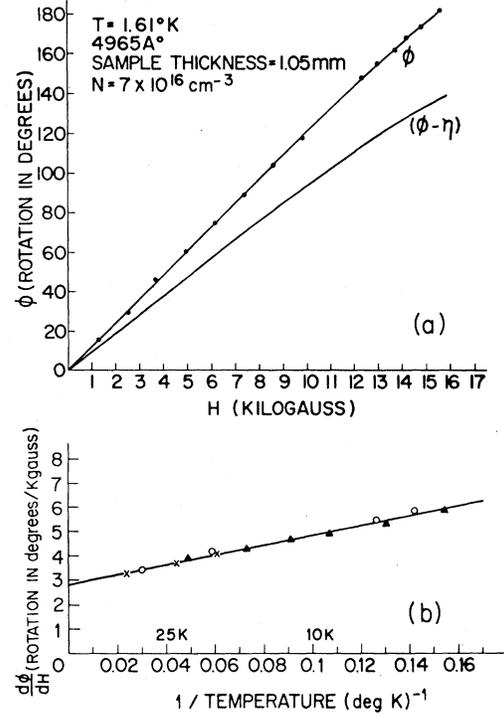
FIG. 1. (a) Field dependence of the observed FR,  $\phi$ , at  $4965 \text{ \AA}$  and of  $\phi - \eta$ , the spin FR obtained by subtraction of the temperature-independent part  $\eta$  derived as described in the text. (b) Temperature dependence of  $d\phi/dH$  used to obtain  $\eta$ . Different symbols for data points represent different runs.
