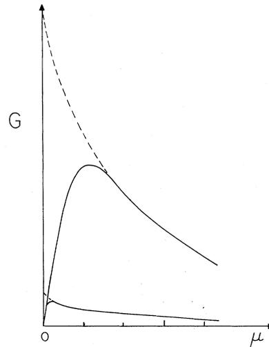
FIG. 2. Temporal behavior of  $g(\mu)$ . The upper curve corresponds to a Doppler width 10 times less than the lower one. The dashed curves represent the evolution of the gain if the finite rise time of the gain is not taken into account.
