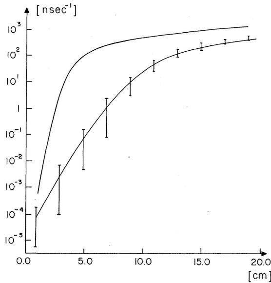
FIG. 1. Energy of the pulse as a function of the length of amplifier. The lower curve represents the actual growth of the pulse, while in the upper curve, the time decay of the gain is not taken into account.
