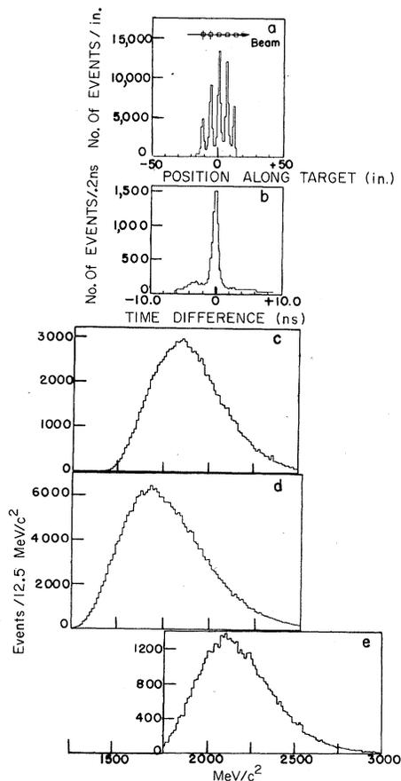
FIG. 1. (a) Reconstruction of the pair vertex at the target, using information from the proportional chambers. The five pieces of beryllium are seen clearly. (b) Time difference between the additional scintillation counters at the back ends of the left and right arms. The resolution obtained is 0.9 nsec and little background is present. (c)–(e) Mass spectra at the lowest mass setting for  $K^+\pi^-$ ,  $\pi^-\pi^+$ , and  $\pi^+K^-$ , respectively.
