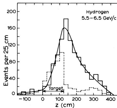
FIG. 2. Decay vertex  $z$  distributions for  $K^0 \rightarrow \pi^+\pi^-$ . The dotted histogram indicates the amount of background subtraction. The solid histogram is the data after background subtraction. The region of the target is indicated. The solid curve is the calculated vertex distribution using the fitted values for amplitude and phase.
