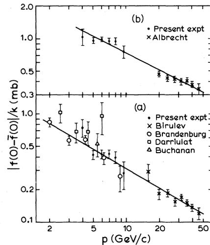
FIG. 4. Regeneration amplitudes for (a) hydrogen and (b) deuterium using average phases of  $-45^\circ \pm 3^\circ$  and  $-39^\circ \pm 4^\circ$ , respectively. The straight lines represent fits of the form  $p_{lab}^n$ .
