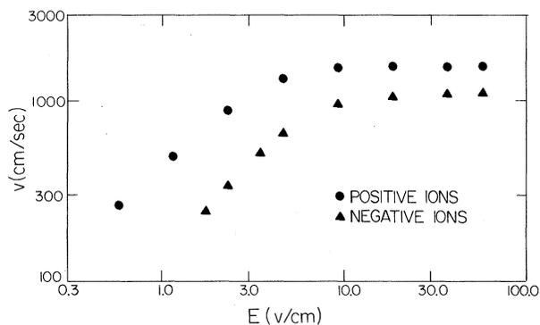
FIG. 2. Electric field dependence of the ion velocity, defined in terms of the leading edge of the ion pulse, at  $T=0.41$  K.
