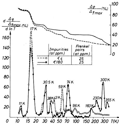
FIG. 1. Isochronal recovery of W after 3-MeV electron irradiation at 4.5 K. Warming rate: 0.1–2 K min<sup>-1</sup> depending on the temperature range. The Frenkel-pair concentration is estimated with  $4.1 \times 10^{-6} \Omega \text{ cm/at.}\%$  (Ref. 7). The impurity concentration is estimated from the residual-resistance ratios ( $\approx 1700$  and  $\approx 70\,000$ ) following Krautz and Schultz (Ref. 8), assuming Mo atoms.
