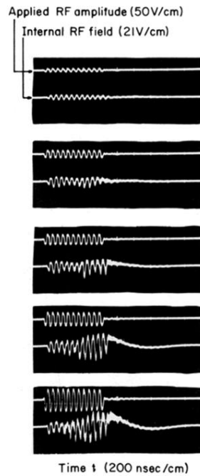
FIG. 3. Temporal plasma response to applied burst at different amplitudes. The lower trace in each picture is the electric field measured by the double T probe located axially in the center of the antenna and radially within the location of maximum density perturbation, i.e., the resonance cone edge. B_0 = 400 G, n_e = 4 \times 10^{10} \text{ cm}^{-3} , f_0 = 15 MHz.
