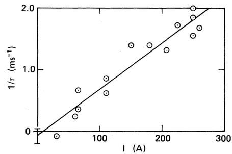
FIG. 2. Density buildup rate versus neutral beam current.
