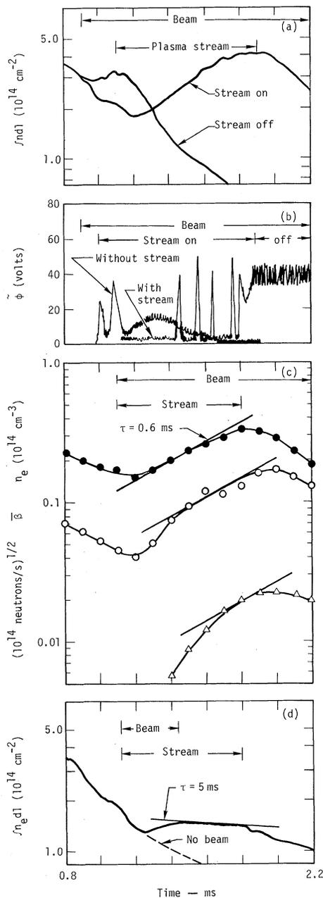
FIG. 1. (a) Line density with and without plasma stream; (b) ion-cyclotron instability amplitude with and without plasma stream; (c) density, diamagnetic-loop, and neutron measurements with plasma stream; (d) line density decay after neutral-beam turnoff with plasma stream.
