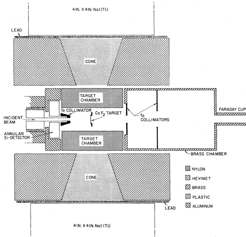
FIG. 1. Scaled drawing of target-detector geometry.
