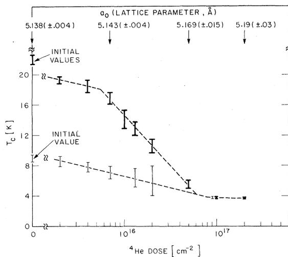
FIG. 1.  $T_c$  versus  ${}^4\text{He}$  dose for films with starting values of 22 and 9 K;  $T_c$ 's are onset and completion temperature ( $\pm 0.2$  K) of resistive transition. Lattice constants of the 22-K films as a function of dose are also shown.
