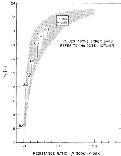
FIG. 2. Resistance-ratio correlation band for 130 as-grown films with the values for damaged films superimposed.
