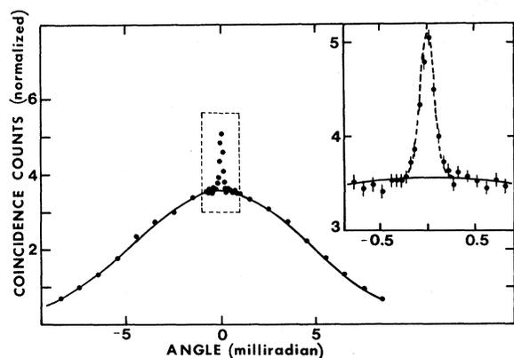
FIG. 2. Angular correlation of photons from positrons annihilating in a single crystal of quartz at  $4.2^\circ\text{K}$  with the  $x$  axis in the direction of measurement. The narrow peak has a width which corresponds to a free positronium atom with a temperature of  $10^{+2}_{-5} \text{ }^\circ\text{K}$ .
