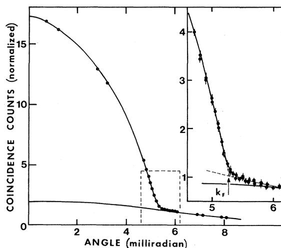
FIG. 1. Angular correlation of photons from positrons annihilating in a Mg single crystal at 4.2°K with the  $c$  axis in the direction of the observed component of momentum. The inset shows an enlarged region near  $k_F$ . The observed slope of the cutoff, the higher-momentum component shown beyond  $k_F$ , and the Gaussian fit to smearing are all discussed in the text. The smearing corresponds to a free-positron temperature of  $10 \pm 10^\circ\text{K}$ .
