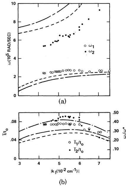
FIG. 3. (a) Measured Alfvén- and drift-mode dispersion relation showing the coupling near  $\omega^*/k_{||} \approx v_A$  and comparison with theory [Eq. (1)] for  $n_e = 5.0 \times 10^{13} \text{ cm}^{-3}$  and other conditions and symbols the same as given in Fig. 2(b). (b) Measured Alfvén- and drift-mode non-linear saturated amplitudes compared with theoretical linear growth rate of coupled drift-Alfvén mode.
