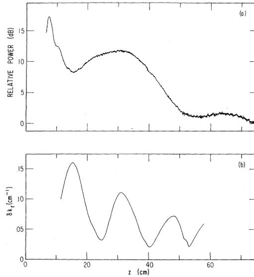
FIG. 2. (a) The wave power and (b)  $\delta k_r(z)$  for the data of Fig. 1(e).
