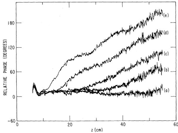
FIG. 1. The relative phase as a function of position. The transmitter is at  $z=0$ .  $\omega/2\pi=135$  MHz,  $k_r=1.83$   $\text{cm}^{-1}$ ,  $e\Phi/T$  is (a) 0.0075, (b) 0.067, (c) 0.16, (d) 0.33, (e) 0.56.
