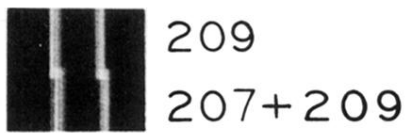
FIG. 3. Spectrogram of the ^{207}\text{Bi} 3067-Å line showing resolved ^{209}\text{Bi} contamination (component f' , identified in Fig. 2) in the radioactive ^{207}\text{Bi} lamp. The weak component c' was also observed, but reproduced only in lower contrast photographs (not shown). The use of an image intensifier decreased somewhat the spectrograph resolution. The ^{209}\text{Bi} reference spectrum is also shown.
