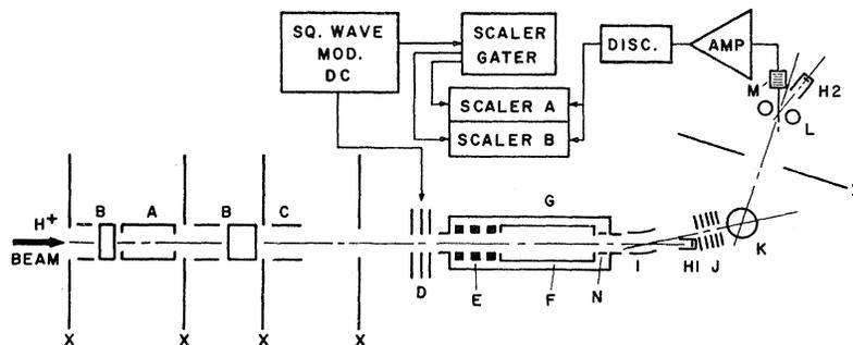
FIG. 1. The merged-beam apparatus: A, electron-transfer gas cell; B, I, L, electrostatic deflection; C, ion-beam gating plates; D,  $n$ -band-defining electric field; E, N, electric-potential change rings; F, voltage-labeled interaction region; G, liquid-He cryopump; H1, H2, Faraday cups; J, electrostatic filter lens [H. D. Zeman, K. Jost, and S. Gilad, *Rev. Sci. Instrum.* **42**, 485 (1971)]; K, deflection magnet; M, particle multiplier; X, differential pumping apertures.
