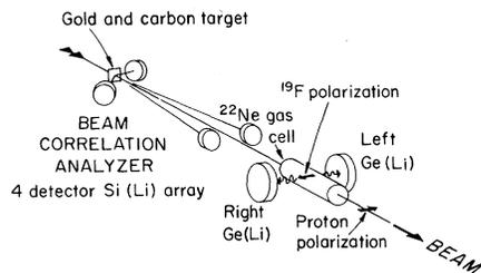
FIG. 1. The experimental geometry is shown. The beam first passes through the beam correlation analyzer which detects changes in beam position, angle, and spin direction associated with the proton-polarization state. Then the beam enters the  $^{22}\text{Ne}$  gas cell where the  $^{19}\text{F}^*$ 's are produced with spins opposite to those of the protons. De-excitation  $\gamma$  rays are detected by the two matched Ge(Li) counters.
