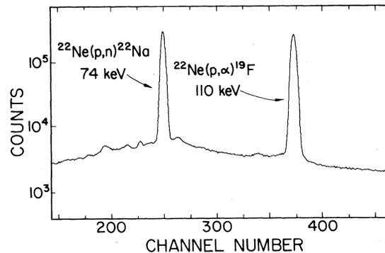
FIG. 2. A spectrum from one of the thin-window Ge(Li) counters showing the good peak-to-background ratio. The smooth background is primarily the Compton plateau of 1.275-MeV  $\gamma$  rays from the  $(p, p')$  reaction.
