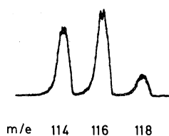
FIG. 4. Mass scan of \text{Br}^n\text{Cl} generated in the thermal reaction (4).
