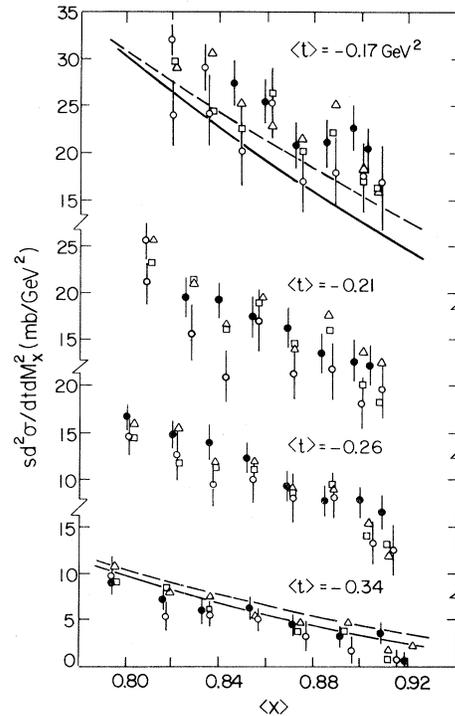
FIG. 3. Inclusive cross sections for the reaction  $pn \rightarrow pX$ . The symbols representing  $\langle s \rangle = 109, 287, 506$ , and  $756$  GeV<sup>2</sup> are as defined in Fig. 1. The solid curves are the sum of the  $\pi\pi P$  and  $\pi\pi R$  contributions to the TR formula (7) with couplings given by Eq. (8). These theoretical curves have been modified, resulting in the dashed curves, to account for Fermi motion and rescattering effects which have not been unfolded from the data.
