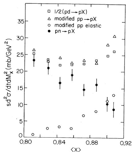
FIG. 2. Sample extraction of  $pn \rightarrow pX$  cross sections from  $pd \rightarrow pX$ ,  $pp \rightarrow pX$ , and  $pp \rightarrow pp$  cross sections at  $\langle s \rangle = 287 \text{ GeV}^2$  and  $\langle t \rangle = -0.21 \text{ GeV}^2$ .
