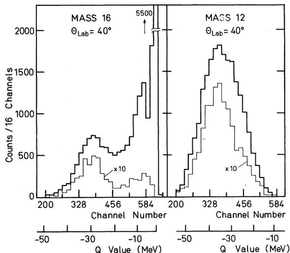
FIG. 1. Energy spectra of mass-16 and mass-12 reaction products from  $^{16}\text{O} + \text{Ni}$  at 96-MeV bombarding energy, both free (heavy lines) and in coincidence with  $\gamma$  rays (light lines). Sixteen channels correspond to 2.0-MeV lab energy, 3800 counts in the free spectra equal 1 mb/sr.
