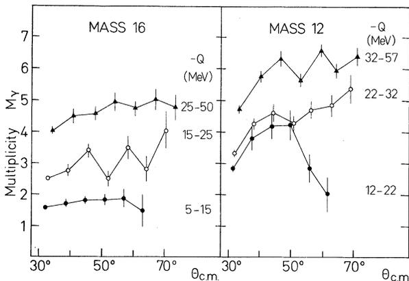
FIG. 3. The  $\gamma$ -ray multiplicity  $M_\gamma$  versus center-of-mass scattering angle for mass-16 and -12 products of different  $Q$  values. Deep-inelastic events (triangles) stand out by having the largest  $M_\gamma$ . Error bars indicate statistical errors only.
