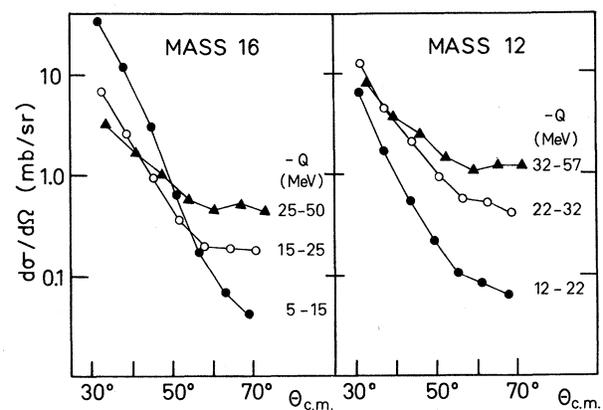
FIG. 2. Differential cross sections versus center-of-mass scattering angle for mass-16 and -12 products for three regions of the spectra, labeled by the  $Q$  values.
