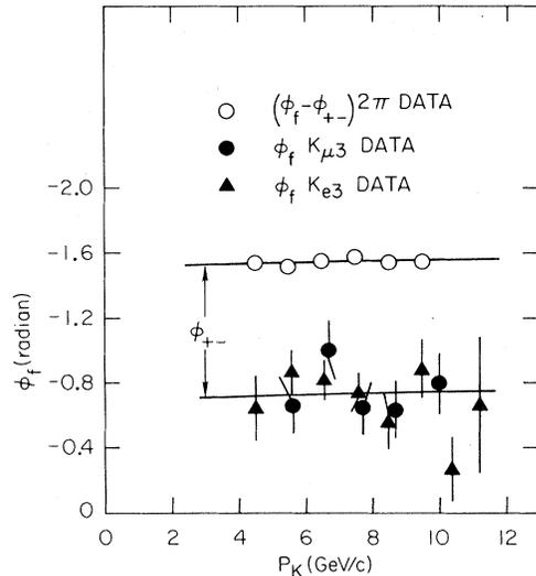
FIG. 3. Results of the combined fit for  $\varphi_{+-}$ . The data points for  $\varphi_f$  are from Table I of the preceding Letter; the  $\varphi_{+-} - \varphi_f$  data are from Table I. The fitting procedure yields two parallel straight lines describing the  $2\pi$  and  $K_{l3}$  data, and whose difference at any momentum is  $\varphi_{+-}$ . The momentum dependence of  $\varphi_f$  is determined almost entirely by the  $2\pi$  data.
