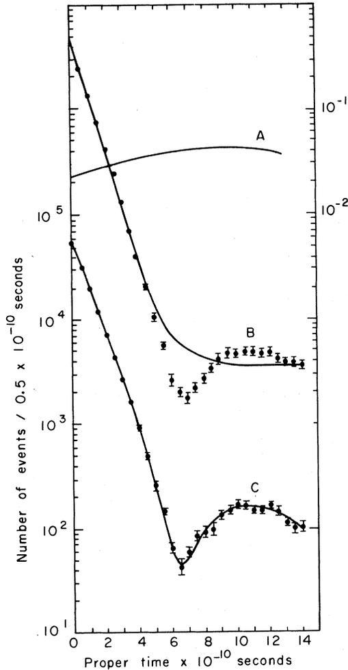
FIG. 1. Curve *a*: The Monte Carlo-derived efficiency for the momentum interval  $5 < P_K < 6$  GeV/c. The absolute value is given by the right-hand ordinate. Curve *b*: Efficiency-corrected data summed over  $P_K$ . The smooth curve is the intensity if  $K_S^0$ - $K_L^0$  interference is neglected. Curve *c*: Data for the interval  $5 < P_K < 6$  GeV/c, uncorrected for the detection efficiency. The smooth curve is the fit of Eq. (5) to the data.
