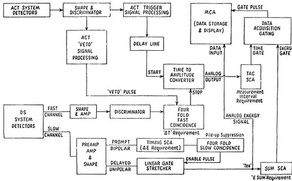
FIG. 2. Block diagram of electronics used for signal analysis and data storage.
