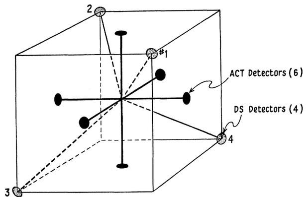
FIG. 1. Schematic representation of geometry for the scintillation counters in the charge-conjugation experiment.
