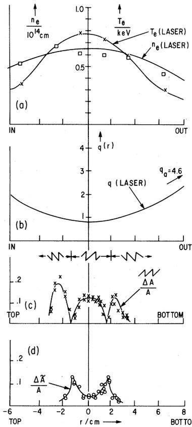
FIG. 2. Radial profiles of (a) electron temperature and density from laser data, (b) the safety factor  $q(r)$  from laser data, (c) amplitude  $\Delta A$  of the internal disruption (sawtooth), and (d) amplitude  $\Delta A$  of the sinusoidal  $m=1$  oscillations preceding the step.
