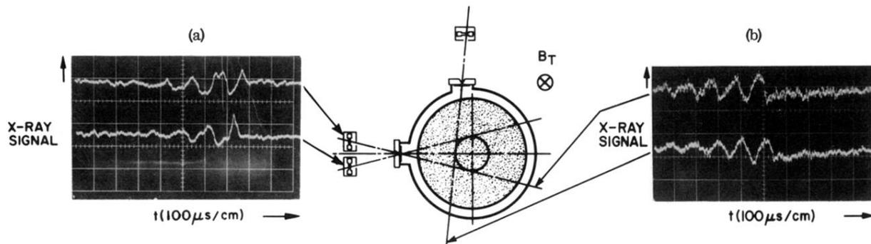
FIG. 3. Determination of  $m$  number of the sinusoidal oscillations. Two detectors look (a) slightly above and below and (b) slightly off center at right angles through the column. The pictures are from different shots. Case (b) shows that the waves go in the direction of the electron diamagnetic drift (i.e., the toroidal field vector  $B_T$  points into the plane of the picture).
