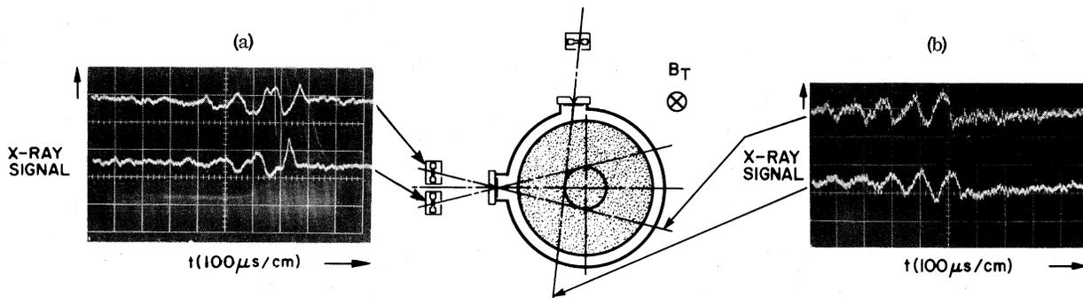
FIG. 3. Determination of  $m$  number of the sinusoidal oscillations. Two detectors look (a) slightly above and below and (b) slightly off center at right angles through the column. The pictures are from different shots. Case (b) shows that the waves go in the direction of the electron diamagnetic drift (i.e., the toroidal field vector  $B_T$  points into the plane of the picture).
