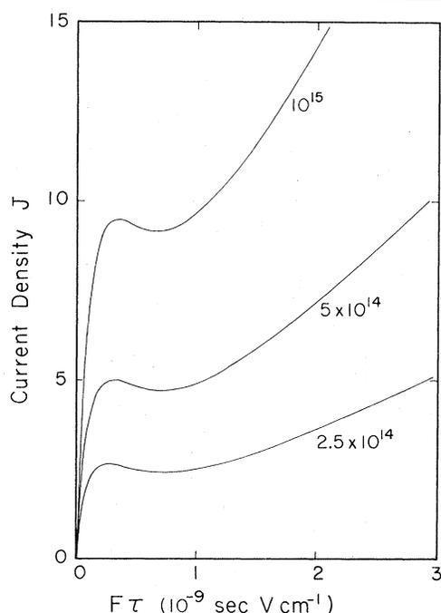
FIG. 3. Average current density  $J$  as a function of  $F\tau$  for samples with different hole concentrations (in  $\text{cm}^{-3}$ ). The current density is expressed in arbitrary units.
