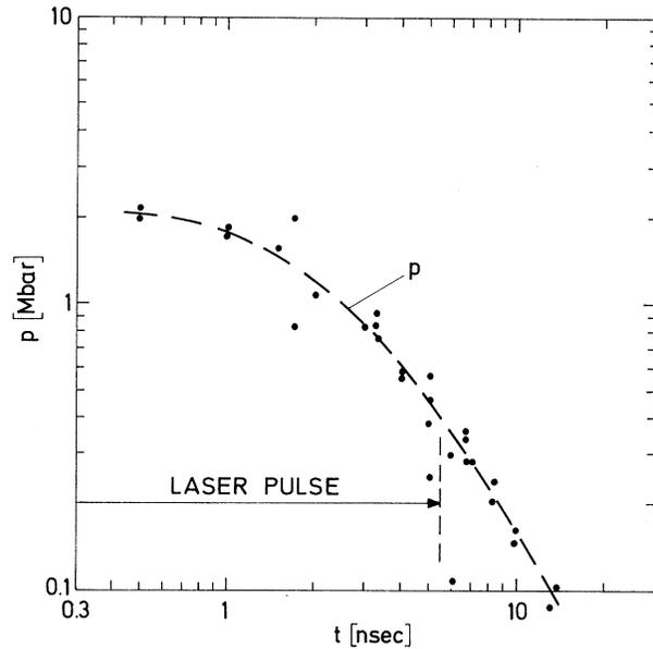
FIG. 2. Pressure  $p_1$  behind the shock wave in solid hydrogen versus time. Data are obtained from five identical shots.
