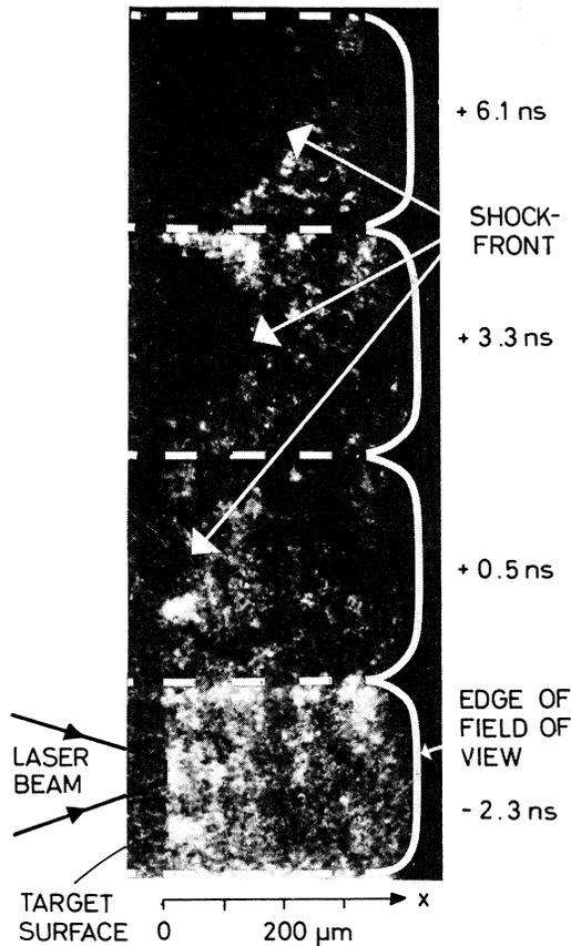
FIG. 1. Framing pictures of a solid-hydrogen target with a mode-locked dye laser as background illumination at 0.5, 3.3, and 6.1 nsec after onset of the laser irradiation.
