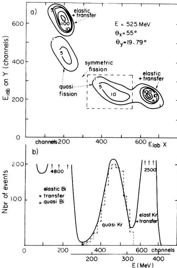
FIG. 1. (a) Two-dimensional distribution (curves of equal numbers of events) of correlated laboratory energies in detectors  $X$  and  $Y$ . (b) Solid line, energy spectrum of all particles (correlated or not) received by the  $X$  detector; dashed line, projection on the  $X$  axis of the quasifission events enclosed in the rectangle of (a).
