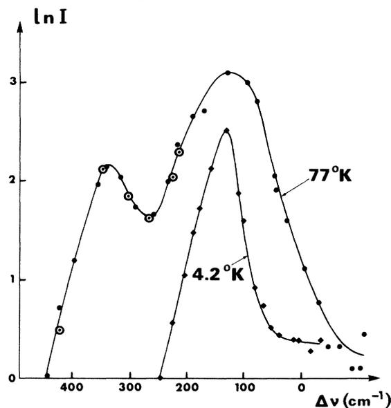
FIG. 2. The two-photon excitation spectrum of CuCl at 77 and  $4.2^\circ\text{K}$ . The natural logarithm of the molecular emission intensity is plotted versus the difference between the  $n = 1$  exciton absorption-line frequency ( $26\,008$  at  $77^\circ\text{K}$ ,  $25\,865\text{ cm}^{-1}$  at  $4.2^\circ\text{K}$ ) and that of the incident light. The open circles are obtained from the direct measurement of  $\delta$ .
