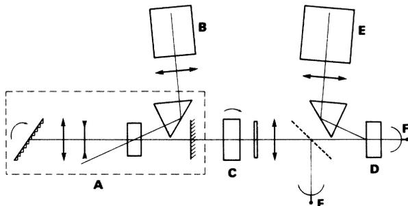
FIG. 1. Experimental setup: A, dye laser; B, ruby laser; C, ADP crystal; D, sample at 4.2 or 77°K; E, monochromator; F, photocell.
