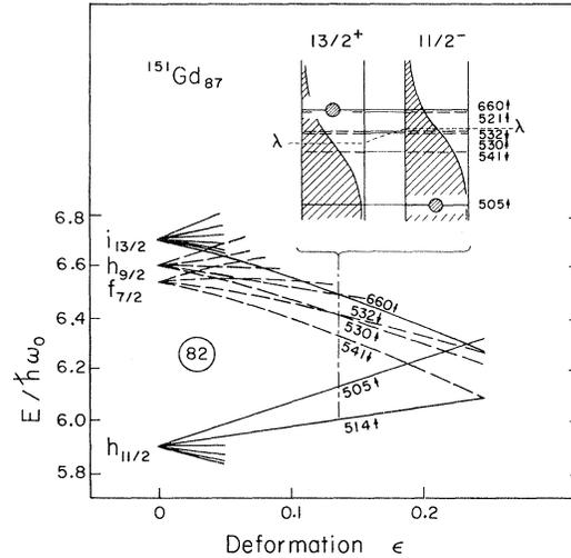
FIG. 3. Nilsson diagram for the  $N = 82$  region. Insets, intrinsic configurations of the  $\frac{13}{2}^+$  and  $\frac{11}{2}^-$  band heads at  $\beta \approx 0.14$ , where the Fermi levels  $\lambda$  are estimated to be those calculated for  $N = 86$  and  $N = 88$ , respectively.
