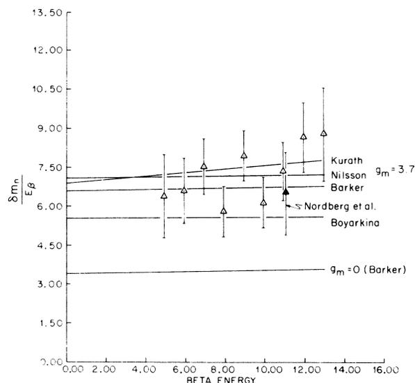
FIG. 2. Experimental results plotted with the wave-function predictions, assuming no second-class current contributions. A datum point from a previous experiment by Nordberg, Morinigo, and Barnes (Ref. 2) has been included to show the good agreement between the two experiments.
