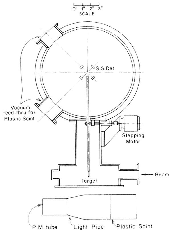
FIG. 1. Vacuum chamber and detector arrangement. Sources produced in the beam are transported, via the stepping motor, into an array of four silicon solid-state detectors and two plastic scintillators. The beam is collimated in order to fix the source location and chopped during the period of rotation.
