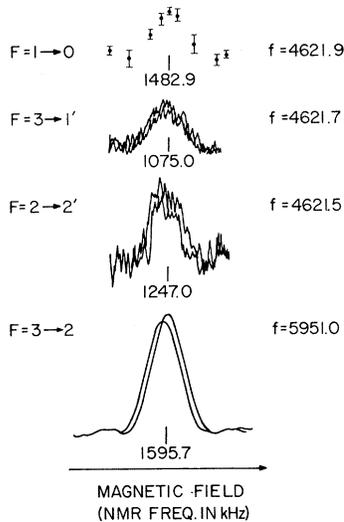
FIG. 4. Zeeman resonance curves for  ${}^3\text{He}^-$ . The magnetic field is shown in units of the proton nuclear magnetic resonance frequency, and the oscillator frequency  $f$  is shown in megahertz.
