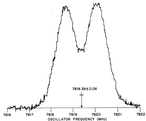
FIG. 3. Resonance curve for the  $J = \frac{3}{2} \rightarrow \frac{1}{2}$  transition in  ${}^4\text{He}^-$  obtained by sweeping the oscillator frequency with  $H=0$ . The dip is due to interference between transitions with  $\Delta M = \pm 1$  and  $\Delta M = 0$ .
