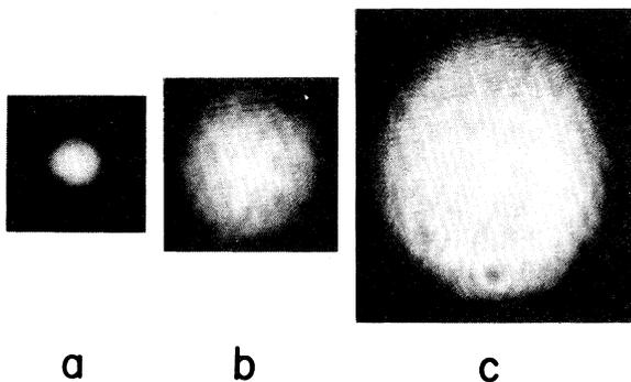
FIG. 2. Far-field patterns of the laser beam after passing through the sodium cell for (a) self-focusing, (b) normal divergence, and (c) self-defocusing.
