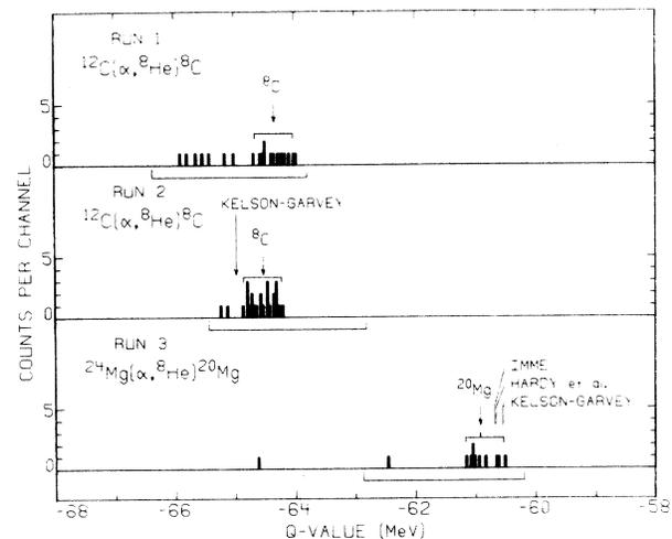
FIG. 2. Spectra of  ${}^8\text{He}$  particles observed in  $\alpha$  bombardments of C and  ${}^{24}\text{Mg}$ , plotted according to  $Q$  value. The channel width is approximately 35 keV. The bracket underneath each spectrum indicates the energy "window" accepted by the magnetic analyzer. In all, 38 events were observed in the ground-state transition to  ${}^8\text{C}$ , and 10 to  ${}^{20}\text{Mg}$ . The theoretical predictions are discussed in the text.
