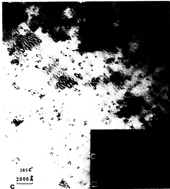
FIG. 1. (a) Background noise from 100-keV electron beam and electron multiplier. (b) Fluctuations in electron multiplier signal which correspond to pretransformation phenomena. The electron current input is the same as for (a) and the horizontal scale is 0.2 sec/cm. (c) Electron micrograph showing streaminglike lattice oscillations in CuAu alloy during pretransformation period.
