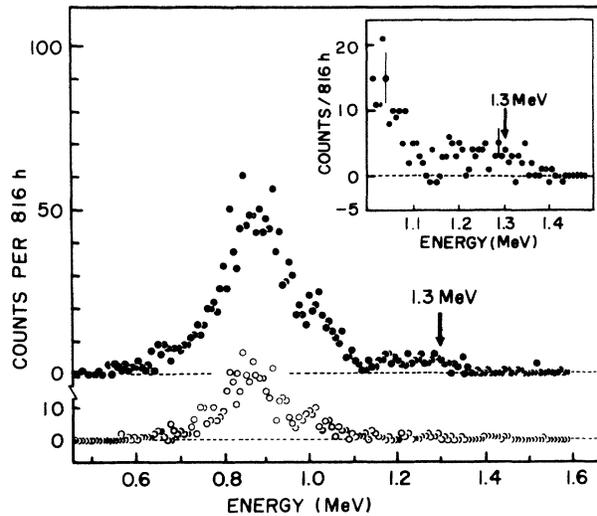
FIG. 2. The observed sum spectrum due to  $K$ -TQA for 300-keV positrons, for the two  $\gamma$  rays emitted at 30 and  $-100^\circ$  with respect to the incident positron direction. The closed circles show a spectrum for Ag, and the open circles show a background spectrum. The inset is the net spectrum obtained by subtracting the background spectrum from the Ag spectrum.
