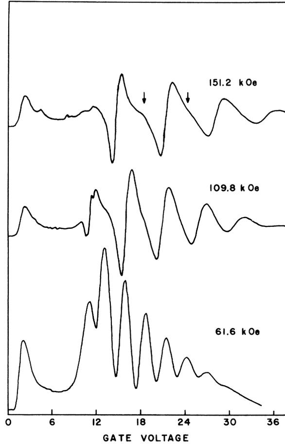
FIG. 1. Transconductance curves at magnetic fields of 61.6, 109.8, and 151.2 kOe. The scale for vertical axis is arbitrary. The horizontal axis shows gate voltage in volts. Arrows indicate the structure in transconductance due to the removal of spin degeneracy.
