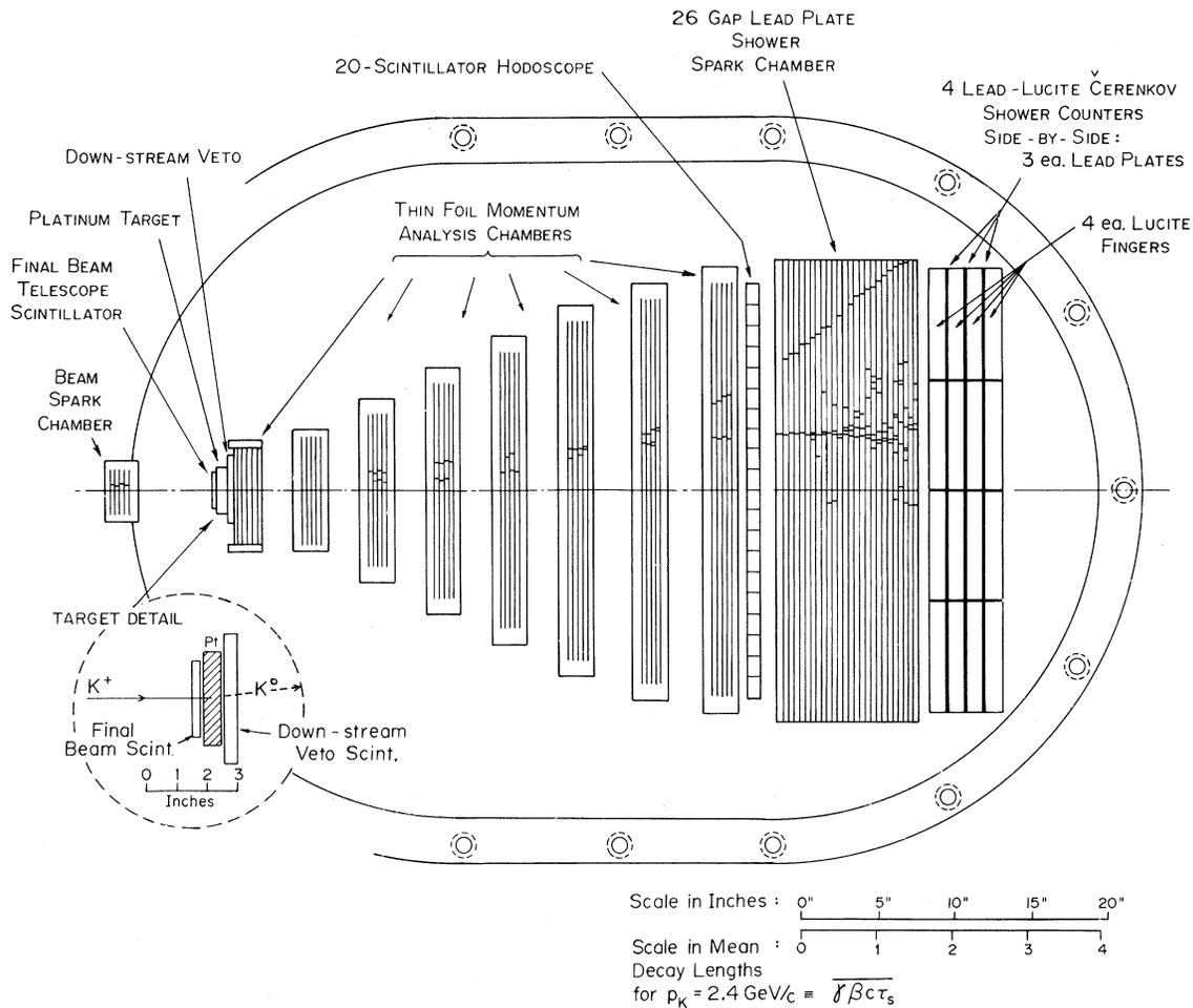
FIG. 1. Schematic plan view of the spark chamber and detector array. The detector array was inside the Argo magnet, whose field was perpendicular to the plane of the drawing. The sparks shown are dubbed in from a real event, but for clarity the side-view mirrors and the images of the sparks in them are not shown.
