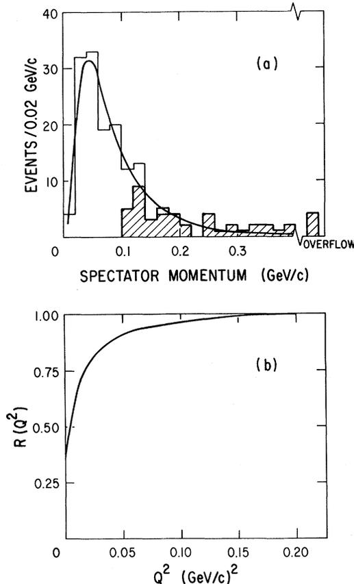
FIG. 1. (a) Fitted spectator-proton momentum distribution. Cross-hatched area, visible spectators; solid curve, Hulthén distribution. (b) Correction factor for the differential cross section to account for the Pauli exclusion principle and Fermi motion in the deuterium nucleus; see Ref. 5.
