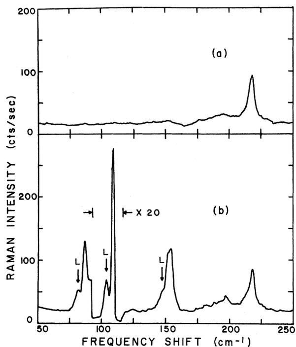
FIG. 1. Raman spectra of  $\text{Cu}_2\text{O}$  at  $4^\circ\text{K}$  with 12 mW incident laser power. Incident polarization,  $[001]$ ; scattered polarization,  $[001] + [110]$ . Instrumental resolution,  $2 \text{ cm}^{-1}$ . (a) Laser frequency  $10 \text{ cm}^{-1}$  above the  $1\text{S}$  yellow exciton frequency. (b) Laser in resonance with the  $1\text{S}$  yellow exciton. The features labeled  $L$  are phonon-assisted luminescence as discussed in the text and in Ref. 2.
