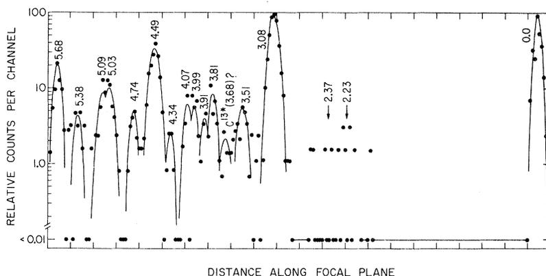
FIG. 1. Spectrum of  $^{48}\text{Ca}(^{14}\text{N}, ^{13}\text{C})^{48}\text{Sc}$  at  $\theta_{\text{lab}} = 22\frac{1}{2}^\circ$ ,  $E_{\text{lab}} = 50$  MeV. This spectrum comprises six individual overlapping position-sensitive detector spectra, each taken at a slightly different spectrometer field setting. These have been normalized to each other, leaving the vertical scale arbitrary.
