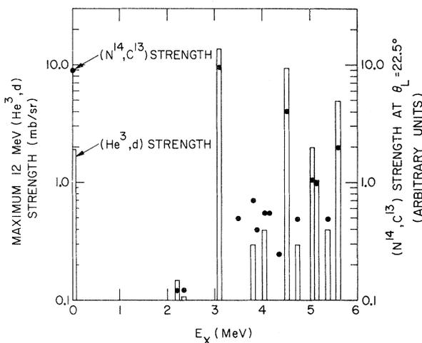
FIG. 2. Comparison of relative yields of levels in ( $^{14}\text{N}, ^{13}\text{C}$ ) and ( $^3\text{He}, d$ ) (see Ref. 5). For those levels seen in both reactions, relative strengths generally match within a factor of 2, except for the ground state,  $\sim 4.5$  times stronger in ( $^{14}\text{N}, ^{13}\text{C}$ ) on this scale.
