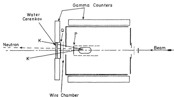
FIG. 2. Rearrangement of the decay system to detect  $K^+K^-$  pairs. For this selection two particles are required in the wire chamber with no signal from the water Cherenkov counter or  $\gamma$  counters. The total ionization in each of scintillation counters P and Q must be near  $4\times$  minimum.
