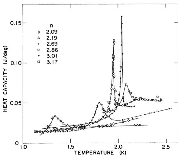
FIG. 1. Reduced-heat-capacity data for coverages up to the filled third monolayer. Solid lines have been added to guide the eye.
