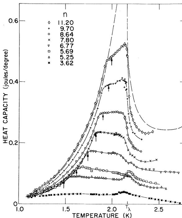
FIG. 2. Reduced heat capacity of multilayer films. Dashed line, heat capacity expected if all atoms above the second solid layer for the film  $n = 11.20$  behaved as bulk. Arrows indicate temperature below which cell relaxation times are immeasurably small. Solid lines are drawn to guide the eye.
