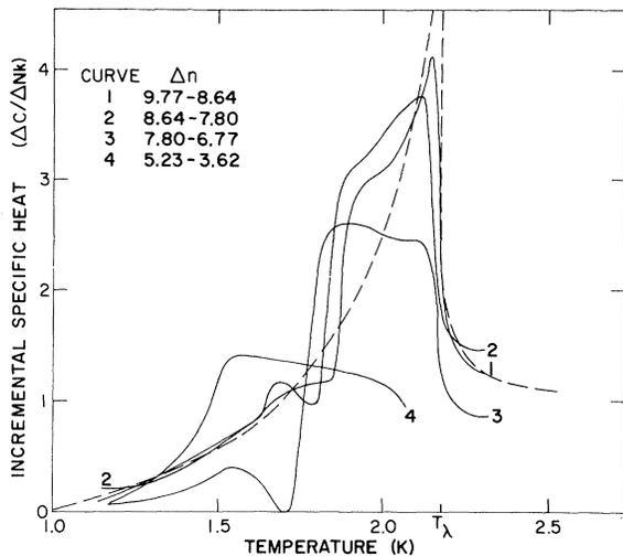
FIG. 3. Incremental specific heat  $\Delta c/\Delta Nk$ , where  $k$  is Boltzmann's constant. These curves are obtained by subtracting smooth fits for adjacent films of Fig. 2. Dashed line, bulk specific heat.
