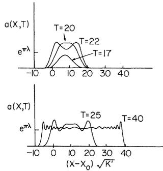
FIG. 1. Temporal evolution of a parametric instability, neglecting damping. A  $\delta$ -function initial value is given at  $x=0$ . In this case  $v_1=5v_2$ , so the instability takes the form of a broadening pulse moving to the right. The initial growth at the point  $x-x_0=(v_1-v_2)t/2$  is given by  $\gamma_0$ .  $\lambda=4$ .
