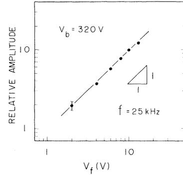
FIG. 3. Wave amplitude versus modulation voltage ( $V_f$ , peak-to-peak value). The ion beam velocity and the frequency are fixed.
