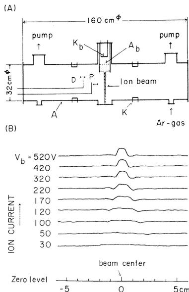
FIG. 1. (a) Simplified experimental setup. Anodes,  $A$  and  $A_b$ ; cathodes,  $K$  and  $K_b$ ; detector,  $D$ ; probe,  $P$ . For ion wave excitation, the ion beams are modulated. (b) Ion current across the ion beams measured with a cylindrical probe, which is 5 cm away from the slit. Zero level is for the ion beam energy  $V_b = 30 \text{ V}$ . The level for a larger velocity is shifted successively.
