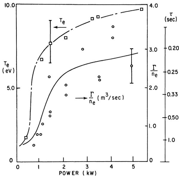
FIG. 3. Electron temperature and loss rate versus input power (bar shows typical experimental error).
