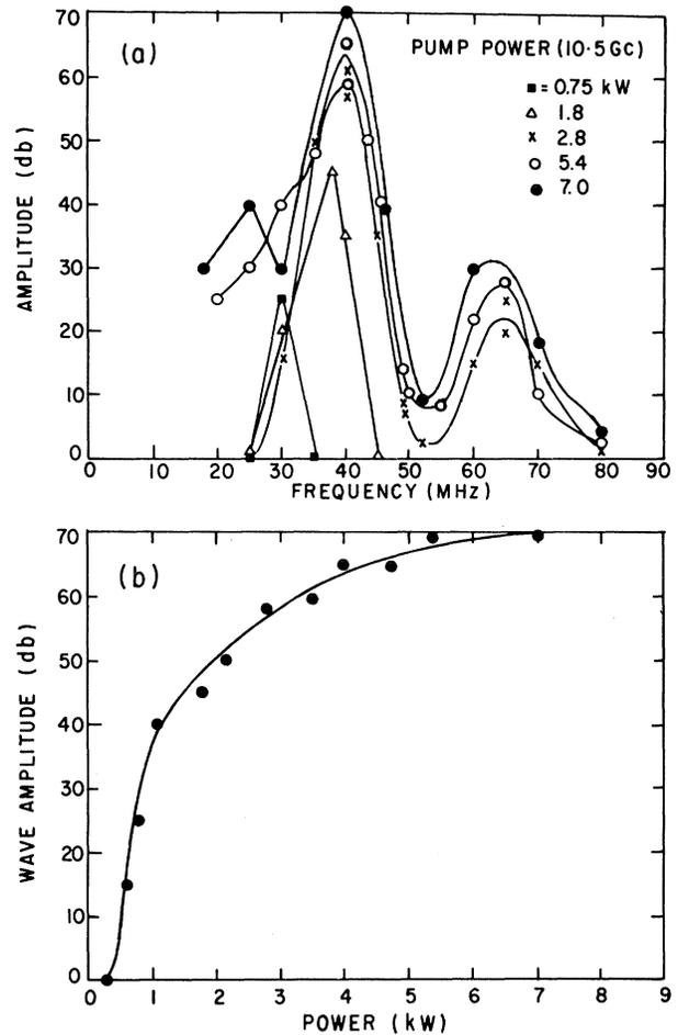
FIG. 2. (a) Frequency spectrum for different input rf powers. (b) Wave amplitude versus input power.
