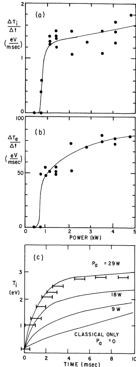
FIG. 1. (a) Heating rate of ion temperature versus input power. (b) Heating rate of electron temperature versus input power. (c) Comparison of time dependence of  $T_i$  with numerical calculations.
