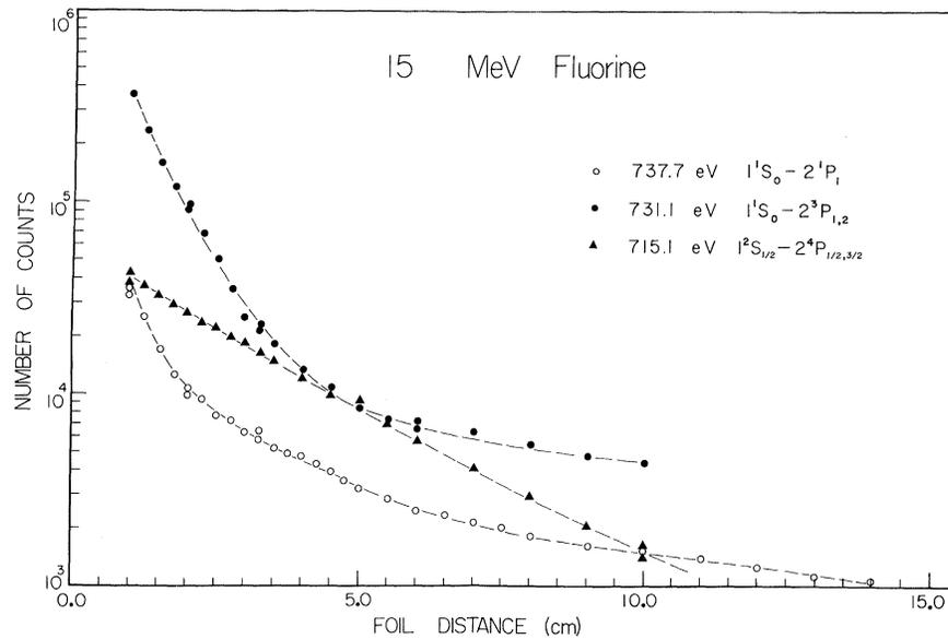
FIG. 2. Decay curves for the three peaks observed downstream from the C foil. The  $2^3P_{1,2}$  curve contains two components with lifetimes of  $\tau_1 = 0.537 \pm 0.02$  nsec and  $\tau_2 = 4.9 \pm 1.7$  nsec. The  $2^4P_{1/2,3/2}$  curve contains one component with a lifetime of  $2.000 \pm 0.025$  nsec.
