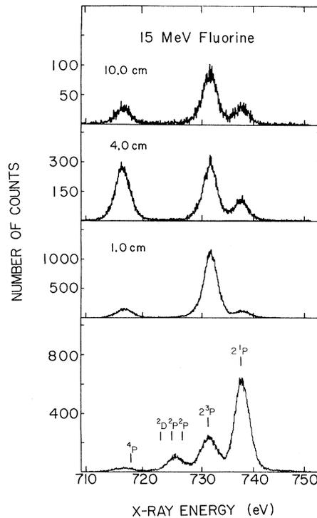
FIG. 1. F x-ray spectra for various upstream foil positions. Bottom spectrum is for a direct look at the carbon foil. Other positions are indicated in upper left-hand corner of each spectrum. The spectra shown here are not all for the same amount of integrated beam.
