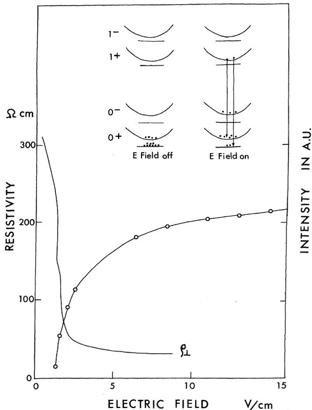
FIG. 3. Resistivity  $\rho_{\perp}$  and peak intensity of the  $1\alpha$  emission as functions of electric field. The inset shows schematically the electron distribution with and without electric field.
