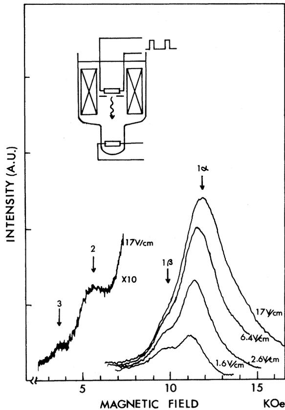
FIG. 1. Intensity of the far-infrared emission at different electric field strengths. The recorder trace in the lower magnetic field side is an enlarged scale to show structures clearly. The inset shows a schematic of the experimental setup. The electric fields indicated are measured at the magnetic field corresponding to the  $1\alpha$  peak.
