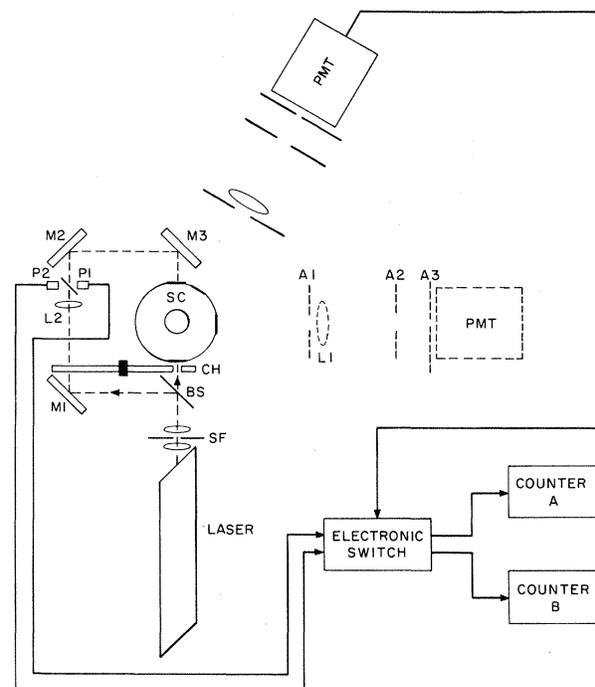
FIG. 1. Diagram of the apparatus used to measure very small anisotropies in the intensity of scattered light.
