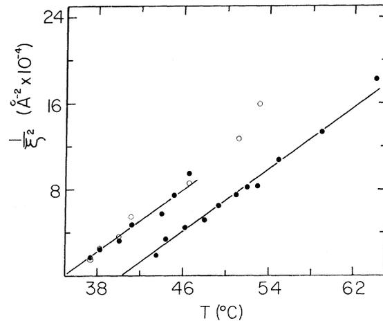
FIG. 2. Reciprocal of the square of the correlation length  $\xi_1$  as a function of temperature in the isotropic phase of MBBA. Data are shown for two samples (see text). Open circles denote corrected data for polarized component. Closed circles denote depolarized component.
