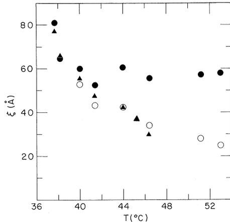
FIG. 3. Functions of temperature in the isotropic phase of MBBA: triangles, correlation length  $\xi_1$ ; closed circles, effective correlation length for polarized light scattering; open circles (see text), corrected correlation length for polarized light.
